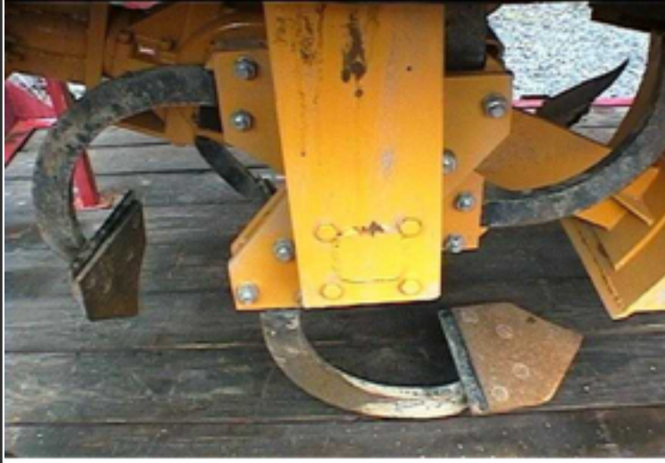
Close-up display of shovels on an Imants spader, a rotating-type spading machine.
