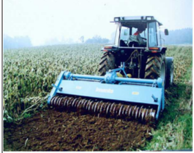
Imants spading machine in the field; working down crop residues in one pass.
